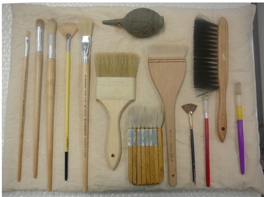
Figure 61: An assortment of brushes (and a photographer's bulb) that can be used for brush vacuuming. Note that the metal ferrule of the brushes (metal section that holds the bristles) should always be covered with masking tape to prevent scratches to the object if accidental contact occurs.
